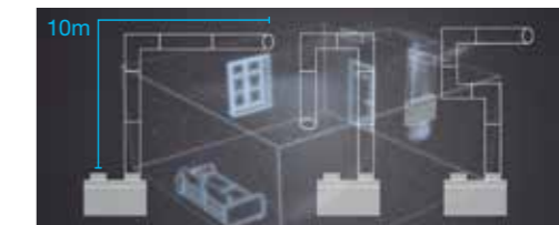
Based on in-house test result, even with a total ductwork length up to 10m, effectiveness of nanoe™ X is maintained.
